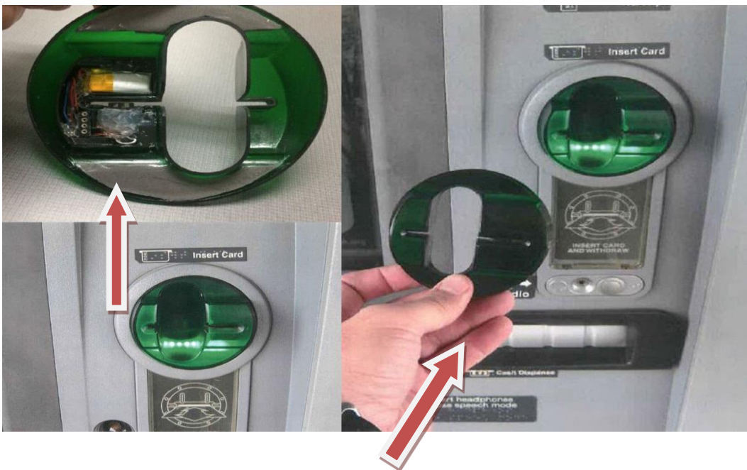
Card Skimmer that is placed at an ATM machine by criminals to copy information
