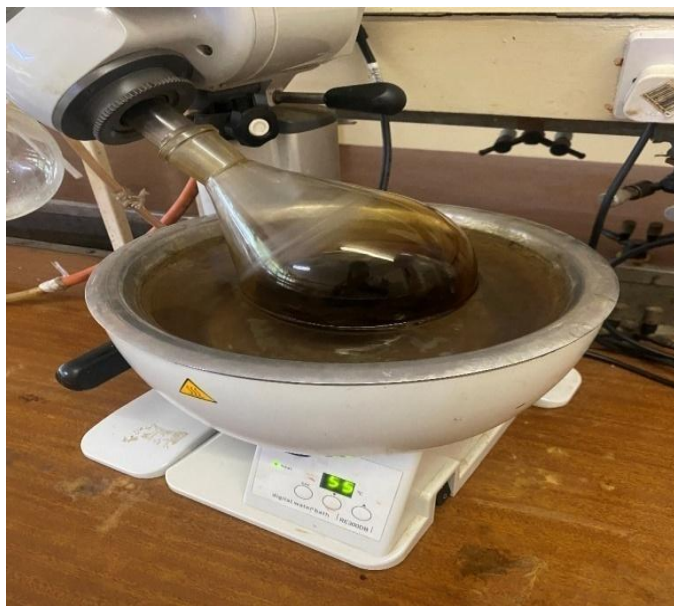
Figure 3.2: A Rotary evaporator (source taken by Tadiwa Muurawa)
