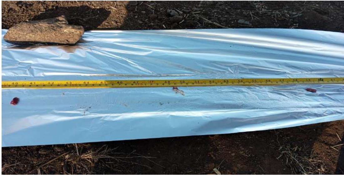
Figure 36: the damaged at speed of 3.41km/hr
