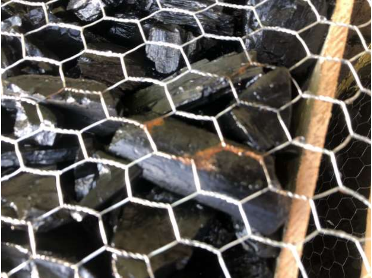
Figure 22: mesh wire reacting with charcoal (rust)
