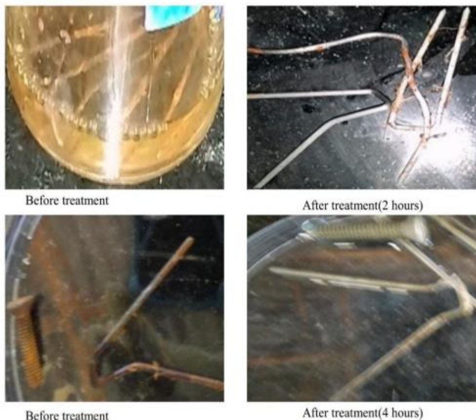
Figure 4.4 Effect of contact time on rust removal (30% phosphoric acid present, pH 1.8)
