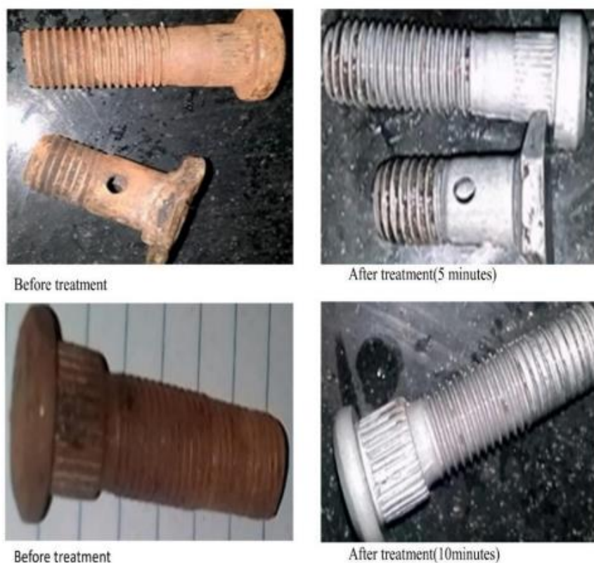
Figure 4.5 Effect of contact time on rust removal 10.2 M
