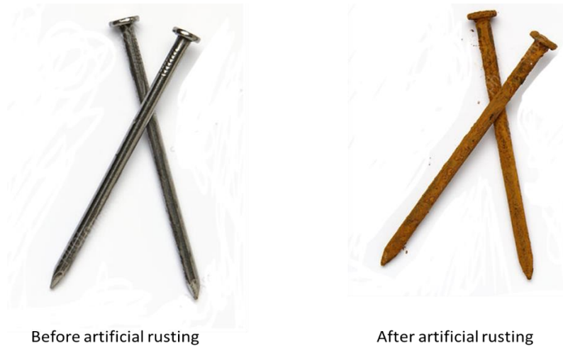
Fig 4.1: Results for artificial rusting
