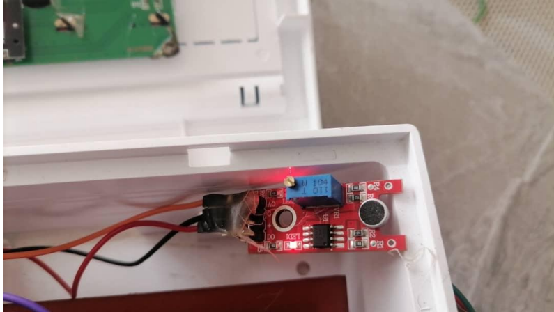
Figure2.1: `microphone positioning in the casing
