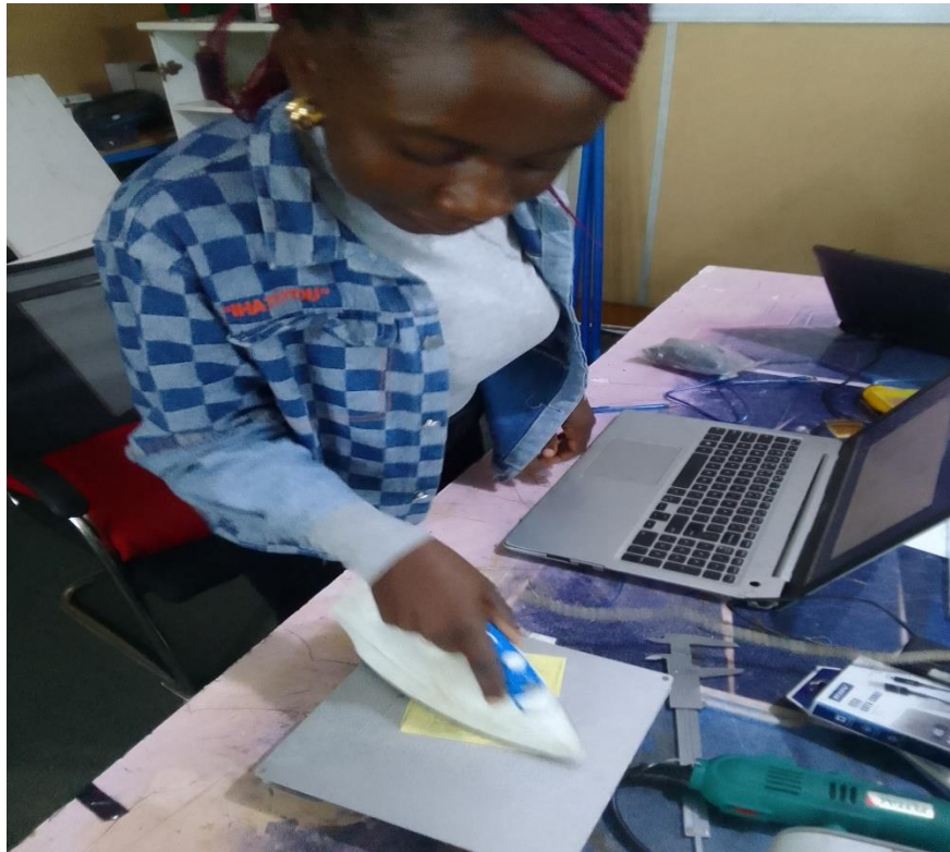
Fig 1.9 shows an image where the author is carefully printing the circuit using a hot iron on the PCB.
