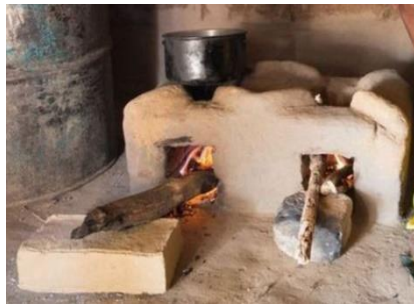
Figure 2.5 : Chingwa stove (Source: http://www.bioenerglis.org )
