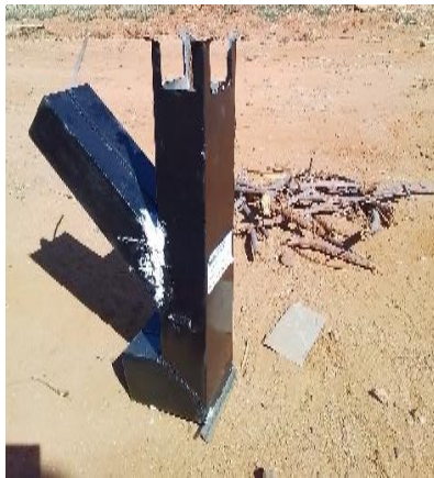
Figure 4.5 : Prototype 1 (Galvanised steel rocket stove)
