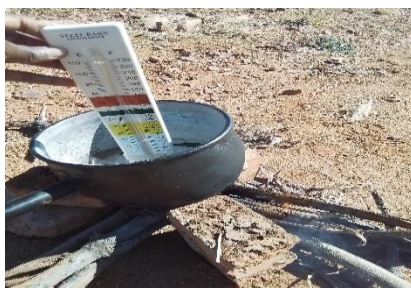
Figure 4.8 : Experimental test 1 process for three stone stove
