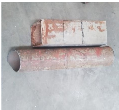
Figure 4.2: Marking angles on desired materials
