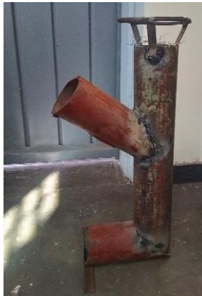
Figure 4.6 : Prototype 2 (Steel rocket stove)
