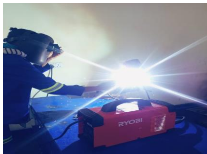
Figure 4.4 : Welding the prototypes using arch welding
