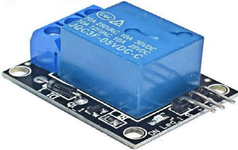
Figure 2.9: image of a JQC3F-05VDC-C relay module used in this project.
