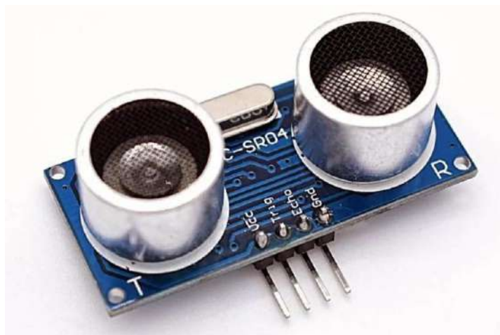
Figure 2.6: image of an HC-SR04 Ultrasonic sensor used in the project for user detection.
