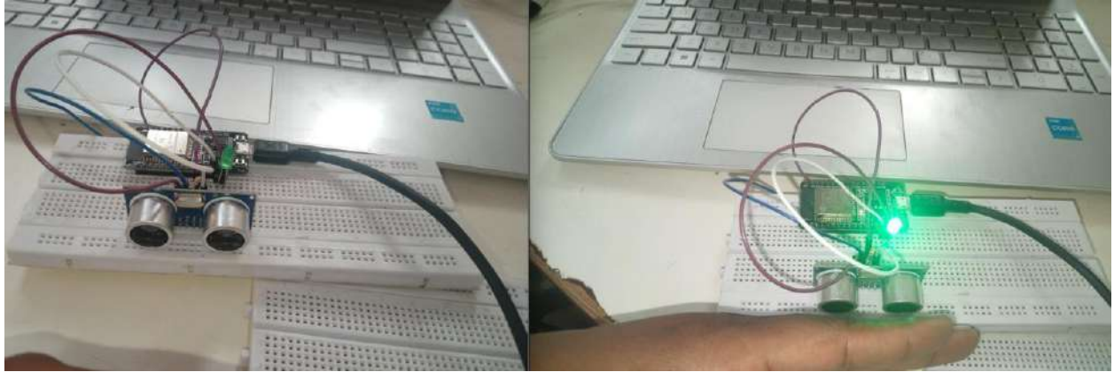
Figure 4.8 Image showing design and testing of ultrasonic sensor detection. Left side shows LED off which shows no user detection and right side shows the LED on which represents user detection within \leq 5\text{cm} range.
