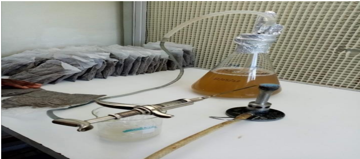
Figure 7. Small scale fermenter for rhizobia inoculation setup in a laminar flow cabinet
