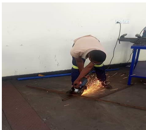
Figure 3.5 Picture showing a student cutting using a cutting disc BUSE workshop
