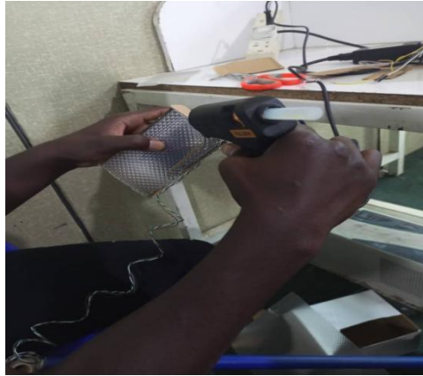
Figure 3.7 The picture showing covering the router for safety reasons using a glue gun.
