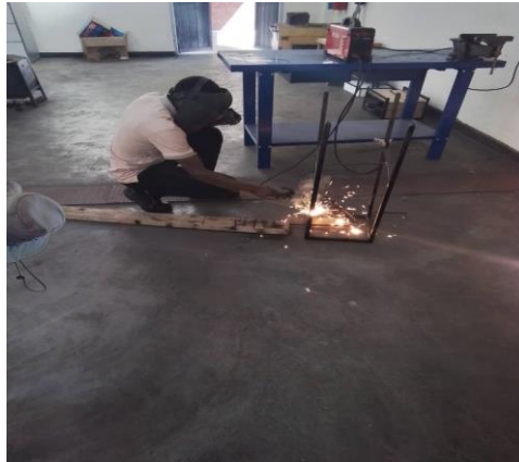
Figure 3.6 Picture showing a student assembly pieces by welding BUSE
