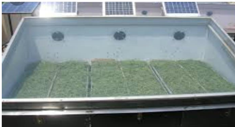
Figure 15 Cabinet solar dryer for green leafy vegetables (Mandisvika et al. , 2015)
