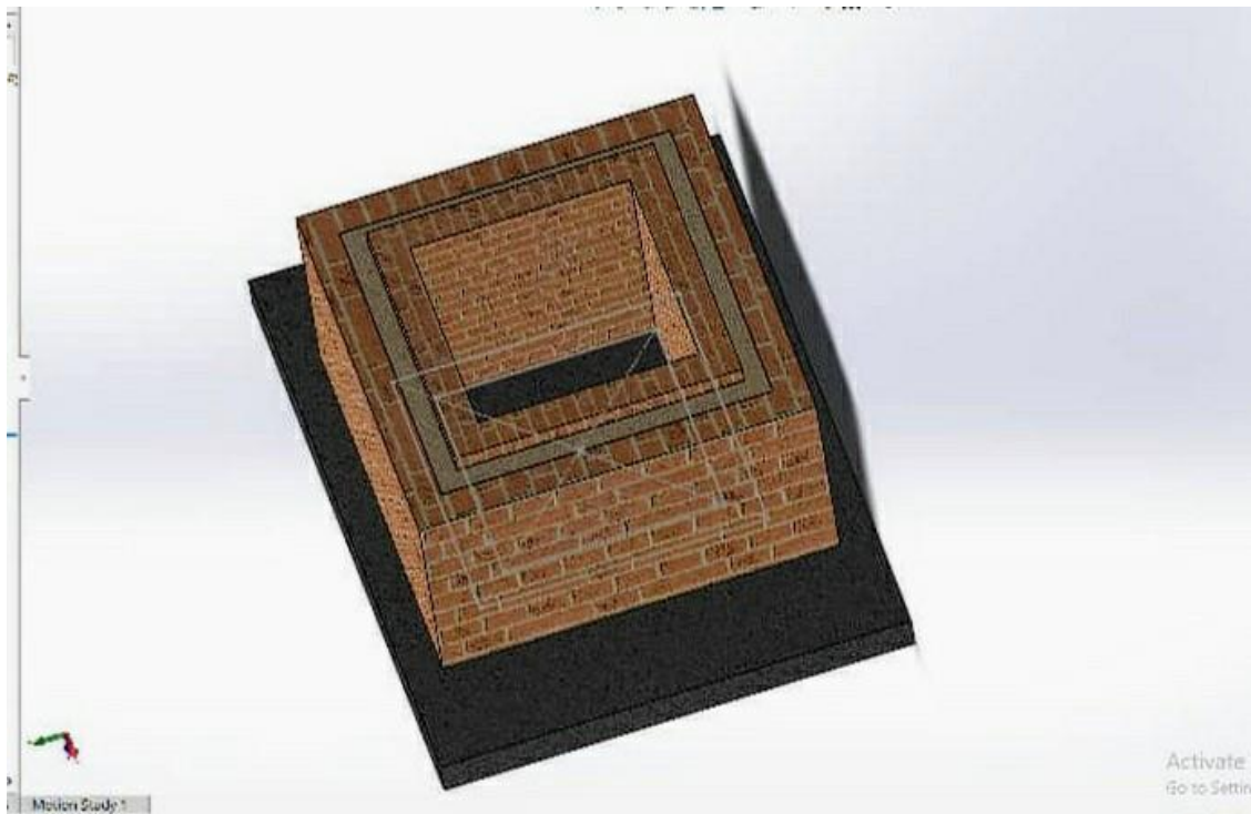
Figure 8: shows an isometric projection of the 3D representation of the ZECC.
