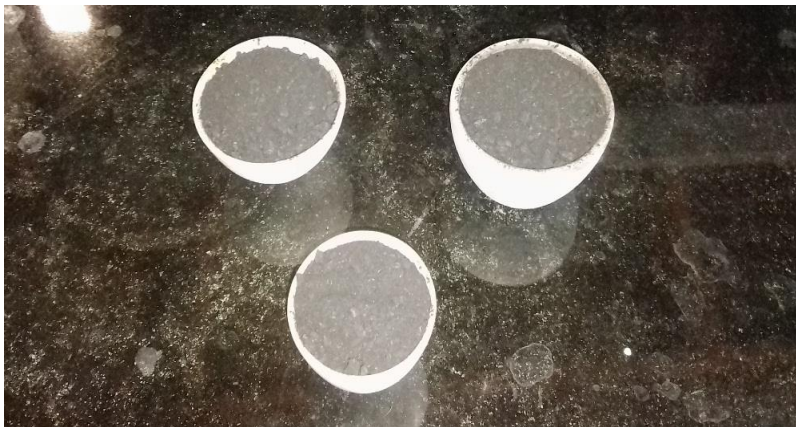
Figure 4.3 Post calcination in muffle furnace at 600°C for 2 hours
