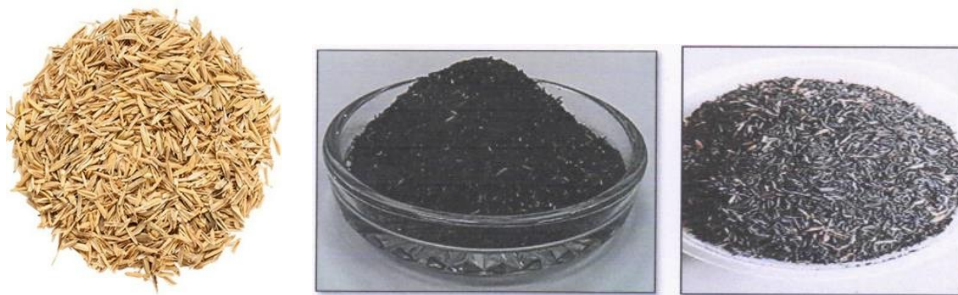
Figure 2.8 (a) rice husk (b) rice husk ash (c) un-sieved rice husk ash
