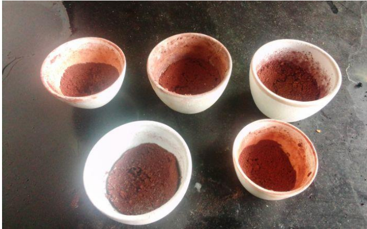
Figure 4.4 Post calcination in muffle furnace at 900°C giving reddish-brown colour
