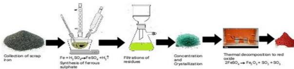
Figure 4: 4 Synthesis step for preparation of red oxide through thermal decomposition of ferrous sulphate
