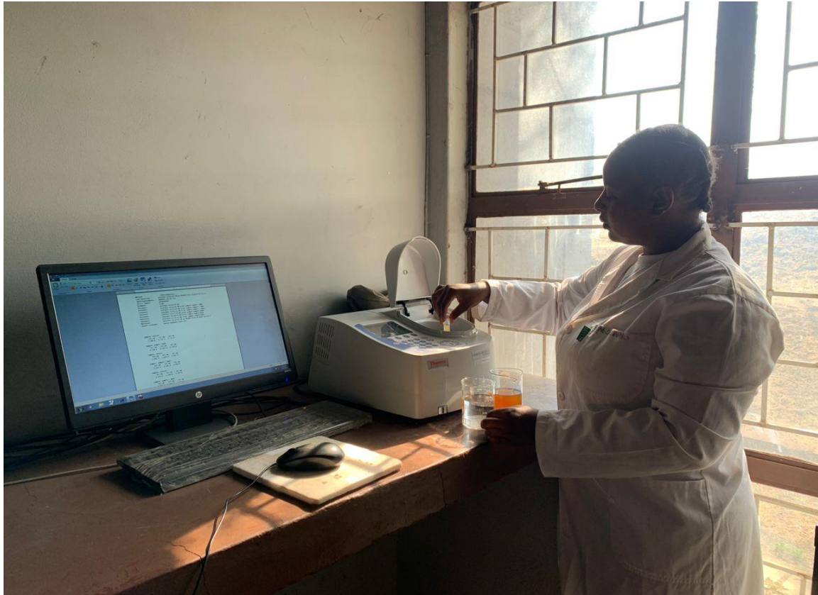
Figure 12: Loading of cuvettes into the UV Visible Spectrophotometer.
