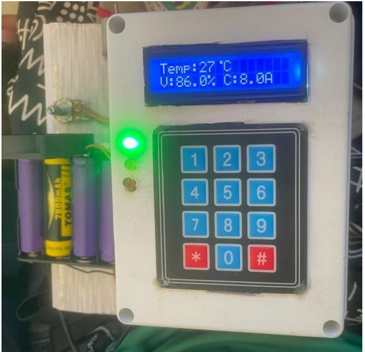
Figure 4.14: LCD testing showing temperature, voltage and current
