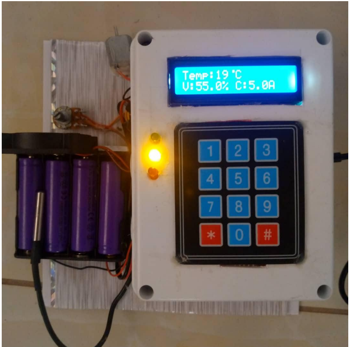
Figure 4.9: Orange LED – Moderate Voltage and Current
