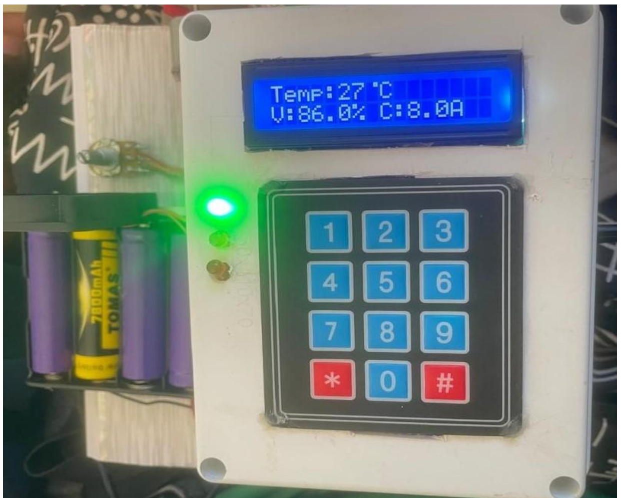
Figure 4.8: Green LED – High Voltage and Safe Current
