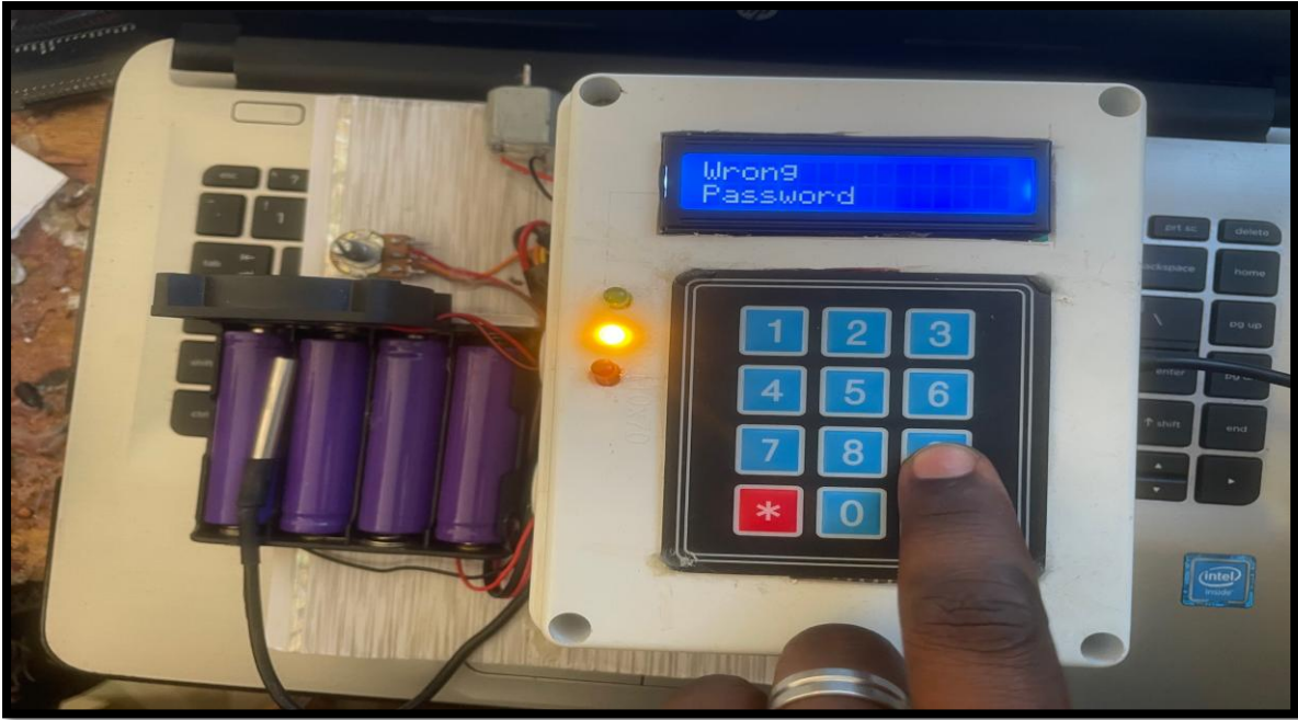
Figure 4.16: LCD Display Showing Password Violation
