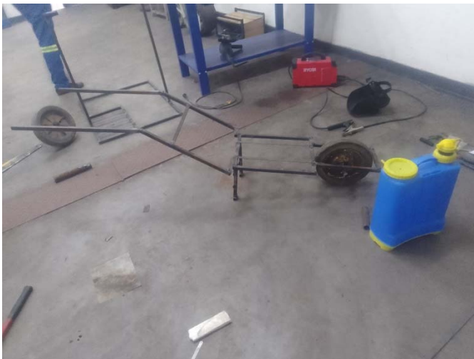
Figure 8: Main frame with wheel
