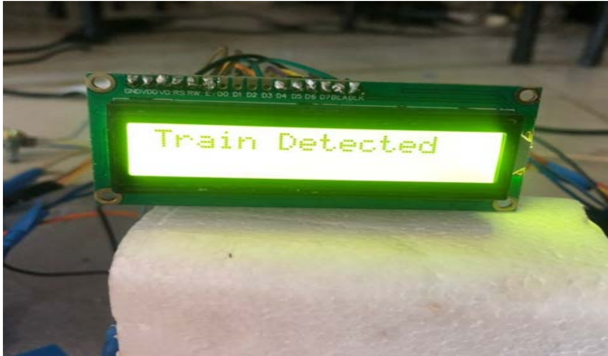
Figure 5.8(a) showing LCD display message when train is detected
