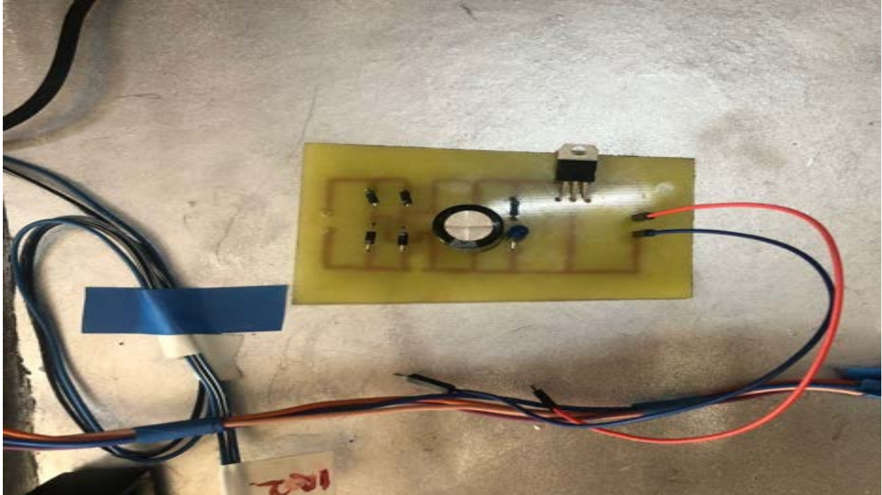
Figure 5.10 showing 5V power supply
