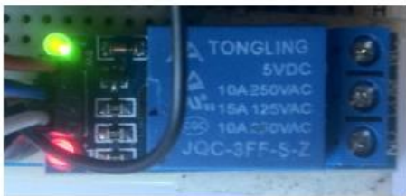
Figure 4-8: relay module activated by hotspot
