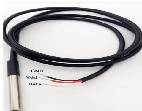
FIG 2.12: DALLAS TEMPERATURE SENSOR
