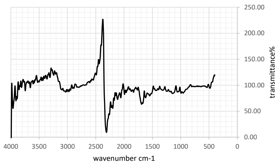
Figure 4.1 FT-IR spectrum of the AC with 60wt% H 3 PO 4
