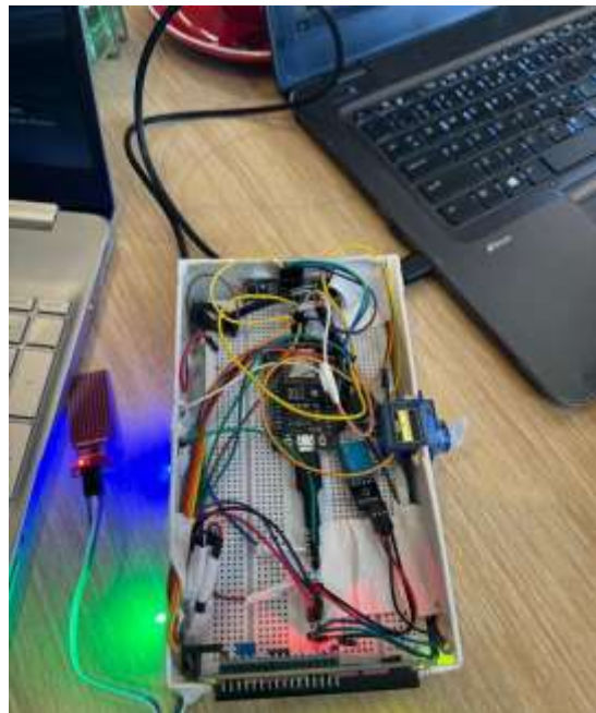
Figure 11: model designed to monitor temperature, humidity and water levels in the coop These components include LCD display.
