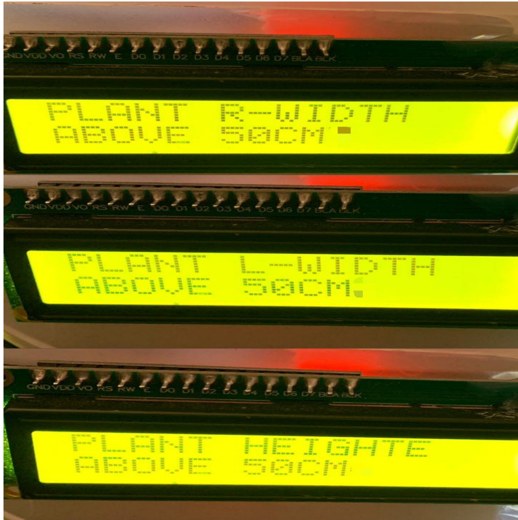
Figure 5.1 system showing the plant height, left and right width of plant triggered display on lcd
