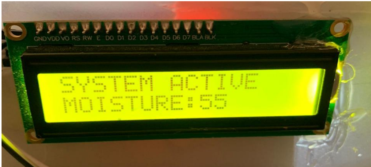
Figure 5.2 shows soil moisture sensor reading on lcd
