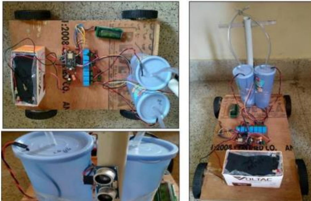
Figure 2.5: A rover to monitor small plant fields
