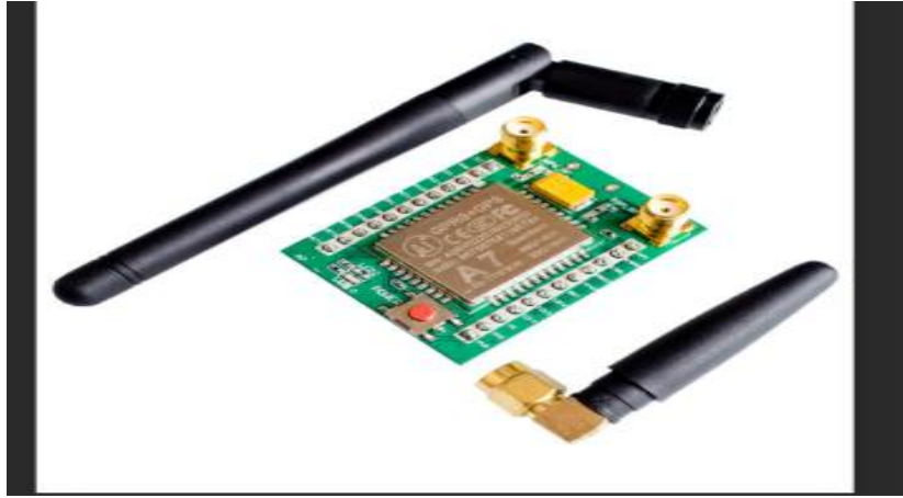
Fig 2.6 [13] Figure shows a Global System for Mobile communication (GSM) module.
