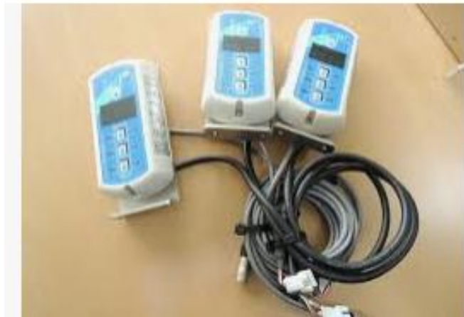
Figure 2.9: Karman vortex flow sensor[8]
