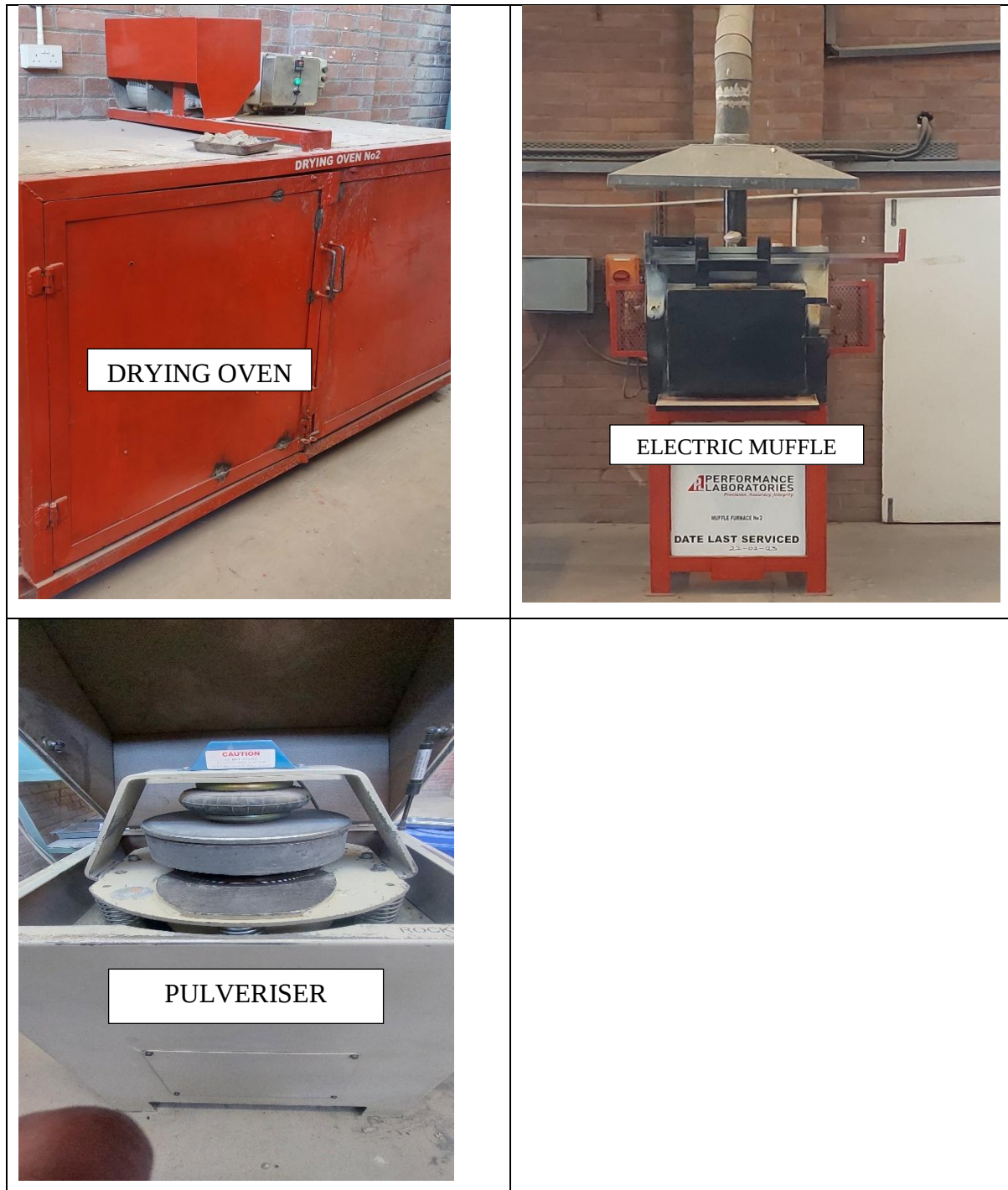
Figure 1: Equipment Used for CCAA Preparation.
