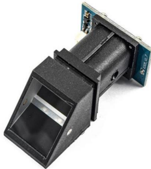
Figure 2.1 : Optical Biometric Fingerprint Reader/Sensor With An R305 Module intended to be used.
