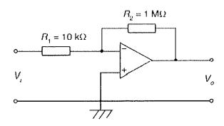
d) For the summing op amp shown in figure below, determine the output voltage,  $V_0$  [3]
