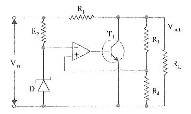
b) The Zener diode in figure below has the following ratings,  $V_z$  = 6.8Vat  $I_z$  = 50 mA,  $r_z$  = 2  $\Omega$  at  $I_z$  = 50 mA,  $I_{z\,(min)}$  = 5 mA,  $I_{z\,(max)}$  = 150mA. What would be the load voltage when the load current  $I_L$  varies from 10 mA to 120 mA. Also, calculate voltage regulation of the regulator. [5]
