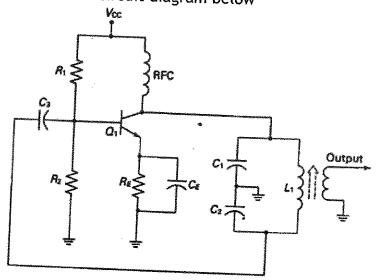
Assume it is desired to design the oscillator so that its oscillating frequency is 4 MHz. If  $\,L_1=\,$  $50\mu H$ , and the feedback fraction  $\beta = \frac{1}{20}$ , calculate
