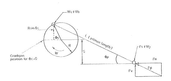
Figure 1: Crank and stoke mechanism
