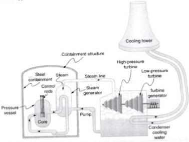
Steam, produced in the steam generator, is used to drive the turbine-generators. Eventually the steam is condensed to water at 27°C and then heated again to start the cycle over.
