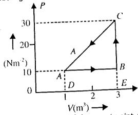
If the internal energy of the gas at point A is assumed zero while at B it is 50 J. The heat absorbed by the gas in the process BC is 90 J. (5)
